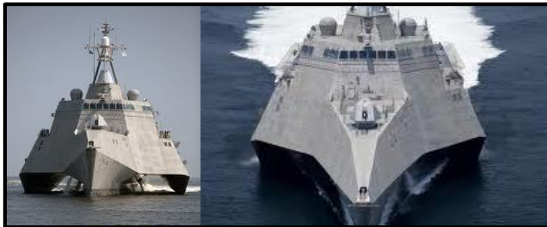
A triple hull ship reduce the interference of waves between hulls reduce rocking
