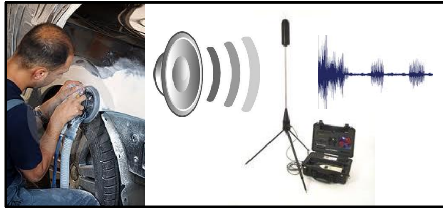
Control of polishing process is done through a speaker. A different sound from the speaker indicates the end of the process
