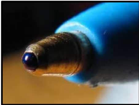
Tiny metal ball rotates at the end of the pen tip – act as cap, enable control flow of ink and avoid clogging
