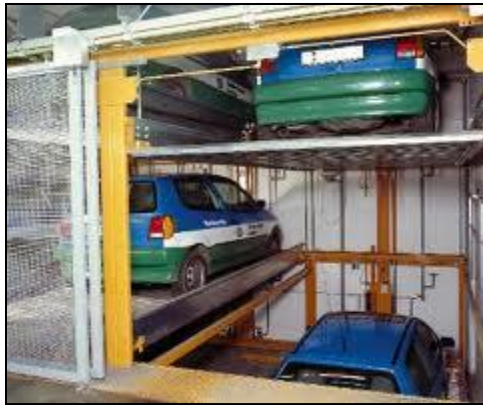
Multi parking system leveraging height dimension to increase capacity
