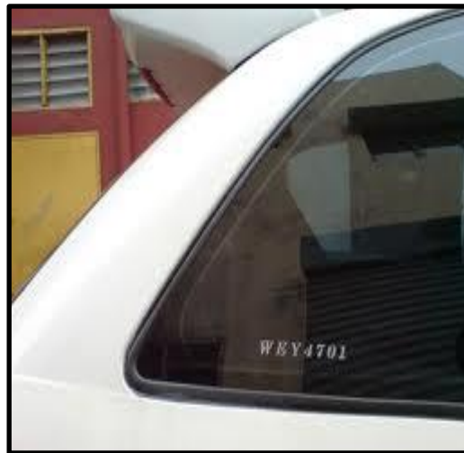
Use sand blasting to create an imprint on glass since both materials are made of silicon
