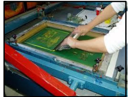
In screen printing, excessive ink is applied on stencil and a squeegee is used to wipe off the excess ink
